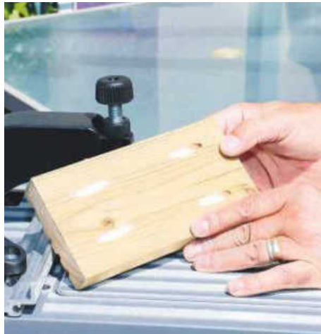
STEP 9. Each board should have four pockets, ready to take the screws
